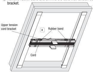
b) Push the **upper tension** cord brackets over the fixing plates until they lock.
