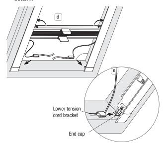
After having checked that the pleated blind functions as prescribed, the excess cord ends can be cut off.
