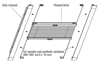
Information: The older window model GGU with 105° mortise requires the spacers supplied to be inserted into the running rail. Place the spacers near the screw.
