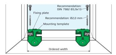
4. Pull the mounting template from the fixing plate.
